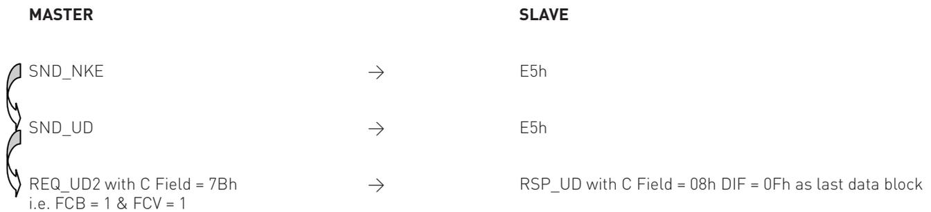
This means that, if the FCB is handled (i.e. FCV = 1), when the RSP\_UD answer has a single-frame of data, the Slave has to send a RSP\_UD answer with the last data block equal to 0F.
