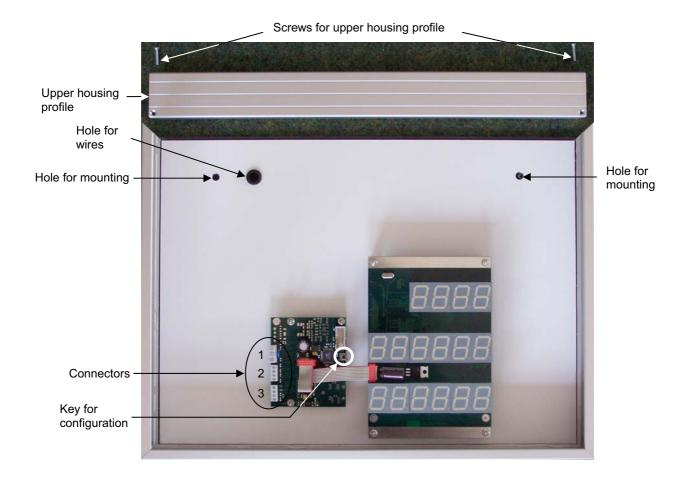
To open the housing of the large display unscrews the upper two screws in the upper housing profile. Remove the upper housing profile and carefully remove the front cover by pulling out to the upper side.
