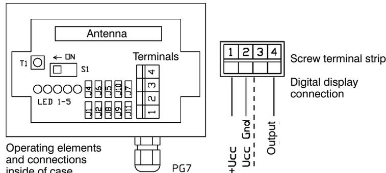
Operating elements and connections inside of case
